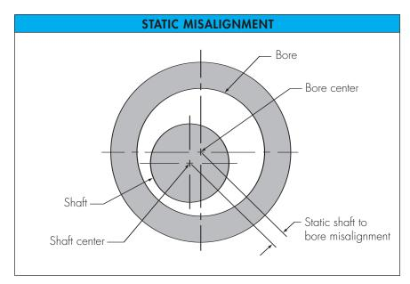
eccentricity increase, the demand on the lip to follow the shaft increases, resulting in shortened seal life. High RPM and eccentricity can cause the seal lip to raise off the shaft, being unable to follow its low point, inducing leakage. Maximum recommended dynamic eccentricity is .005 inches total indicator reading (TIR) or 0.13 mm.
