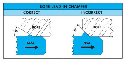
best results. A chamfer of 45 degrees will act more like a snowplow resisting the seal and increasing installation force by more than four times. This high installation force can also cause a hysteresis in the seal's rubber cover resulting in the seal springing back after being seated.
