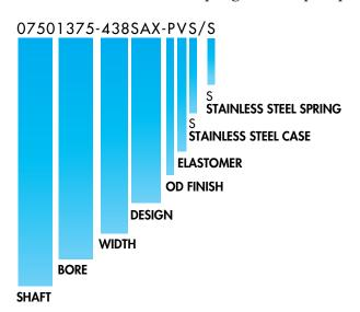
Assume you wish to order Example 2 from page 36 with a stainless steel case and carbon steel spring. The complete part number is:
